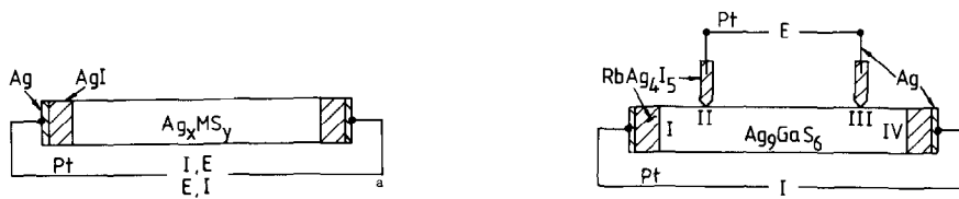
FIG. 1. (a) Two-probe ionic conductivity cell, used in either the constant current or the constant potential mode. (b) Four-probe ionic conductivity cell used for \text{Ag}_9\text{GaS}_6 . Voltage probes II and III measure the potential drop across the sample which is related to the difference in electrochemical potential of silver ions.
